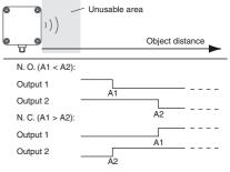
A1  $\rightarrow \infty$ , A2  $\rightarrow \infty$ : Object presence detection Both outputs are active if Object within detection range.
